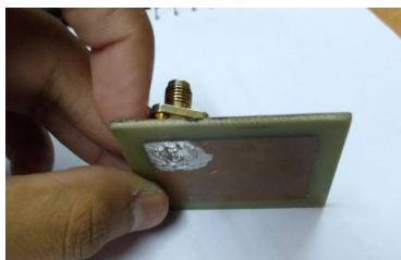
Fig II: Manually Fabricated Patch Antenna
